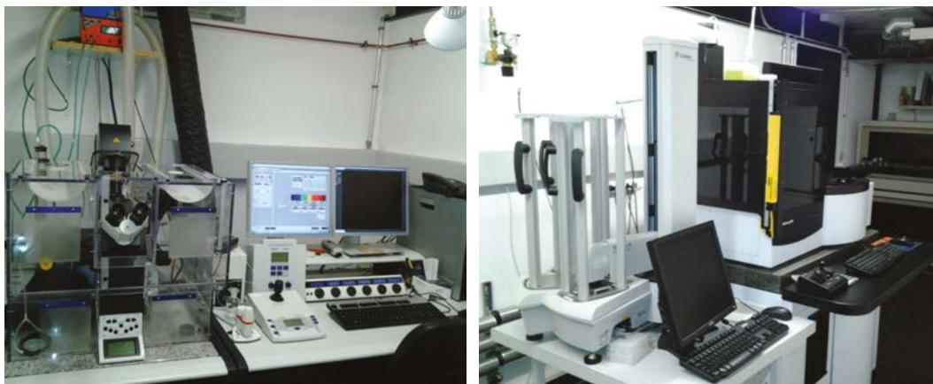
**Figure 1** Left: Confocal microscope *Leica TCS SP5*. Right: High-content screening system *BD Pathway 855*.
